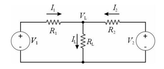
$$V_L = \frac{\binom{V_1}{R_1} + \frac{V_2}{R_2}}{\binom{\frac{1}{R_L} + \frac{1}{R_1} + \frac{1}{R_2}}{}}, I_1 = \frac{V_1 - V_L}{R_1}, I_2 = \frac{V_2 - V_L}{R_2}$$
