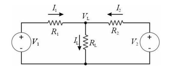
$$V_L = \frac{\binom{V_1}{R_1} + \frac{V_2}{R_2}}{\binom{\frac{1}{R_L} + \frac{1}{R_1} + \frac{1}{R_2}}{}}, I_1 = \frac{V_1 - V_L}{R_1}, I_2 = \frac{V_2 - V_L}{R_2}$$
